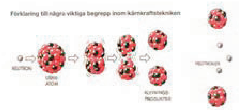
Figure 4-2. Schematic illustration of the fission process. A neutron is captured by a uranium atom, which becomes excited and is split (fissions) into two parts (fission products). At the same time, a number of neutrons are emitted.
