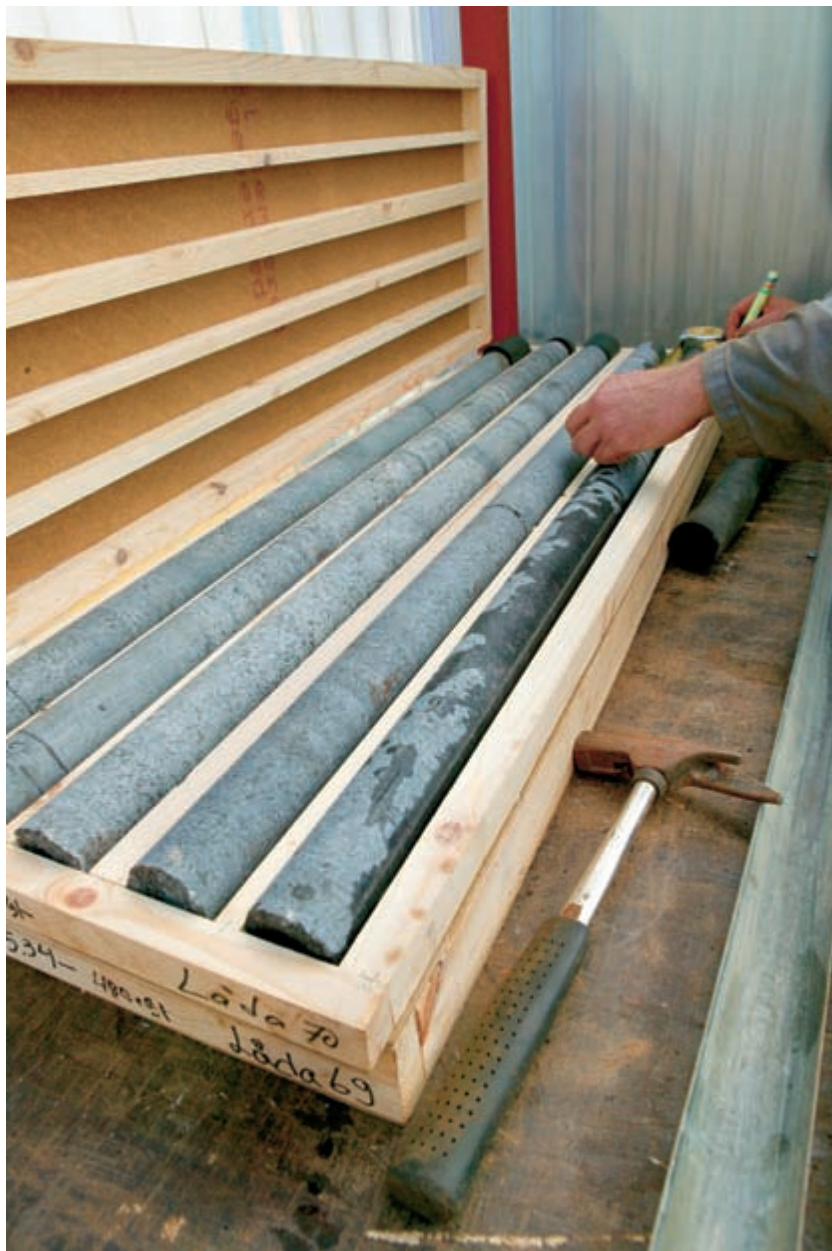
Measurement of drill cores from test drilling. Photo: Carl-Robert Lindqvist. Source: SKB.
